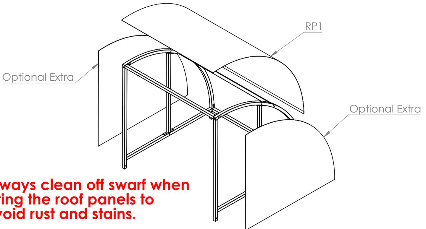
**Always clean off swarf when fitting the roof panels to avoid rust and stains.**
