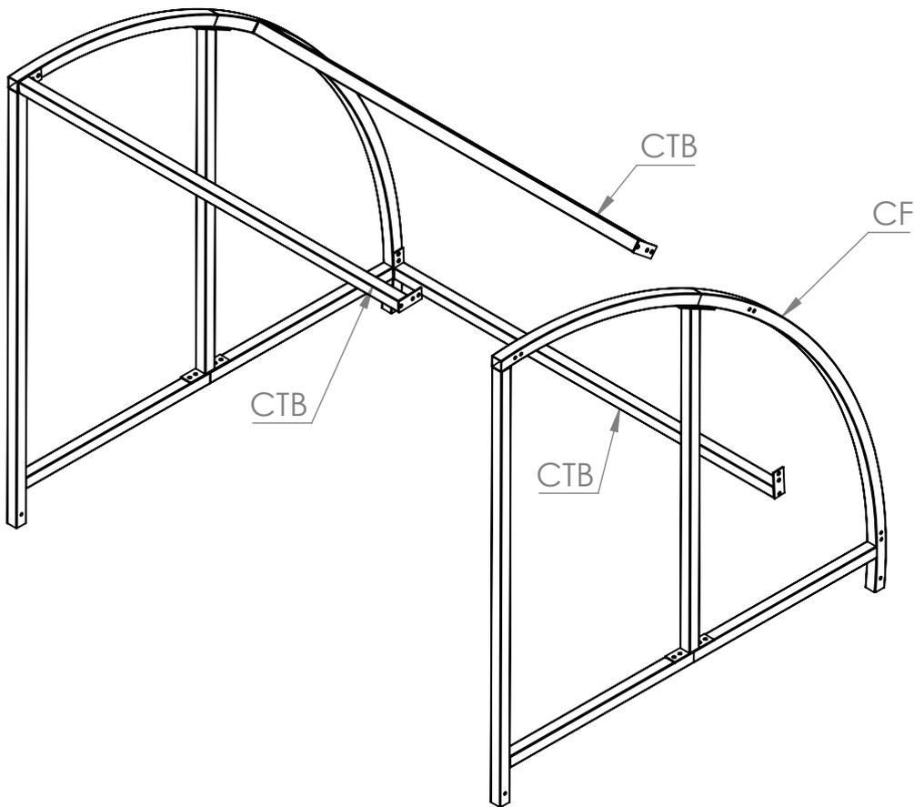
**Step 3** Secure the polycarbonate supplied with the shelter to the outer parameter, using **TEC 25 Screws** in the fixing kit. (Note: 200mm Spacings Between **TEC Screws**)
