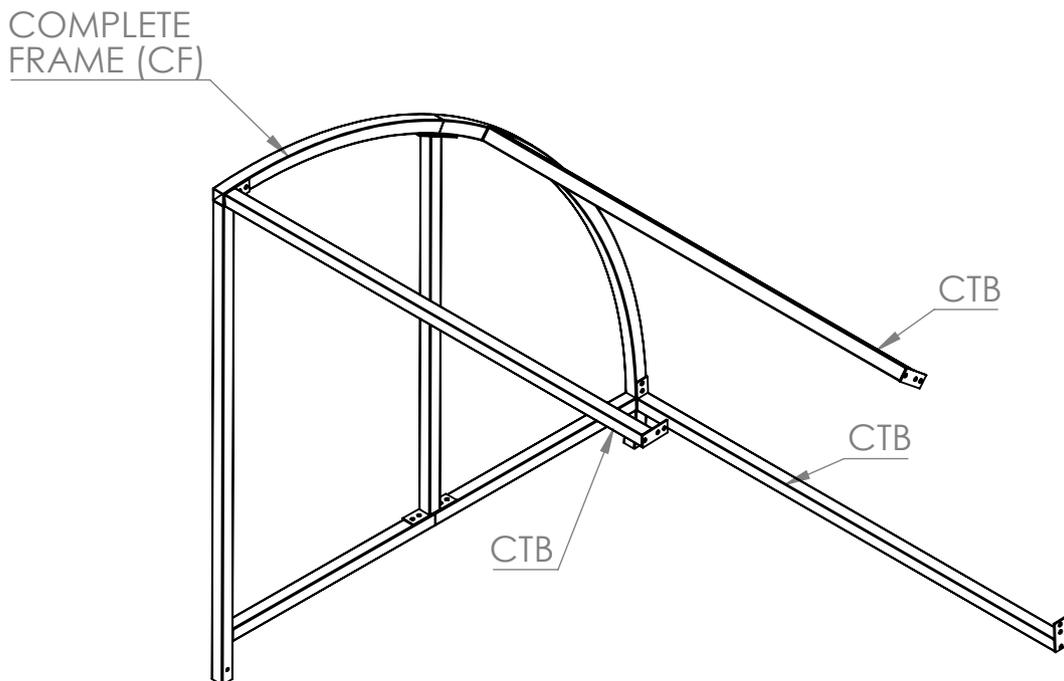
**Step 2** Repeat **Step 1** with the other side of the shelter. (**Structure should now stand without support.**) Make sure all bolts are tight at this point.
