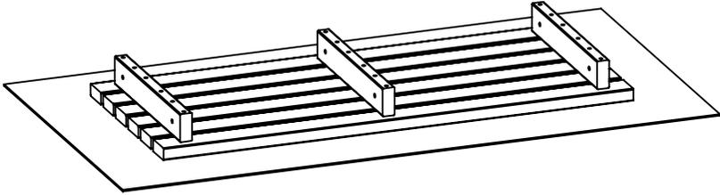
**Step 2** Assemble the A frames by attaching the legs to the cross beams with the nuts and bolts supplied, using 2 washers per bolt.
