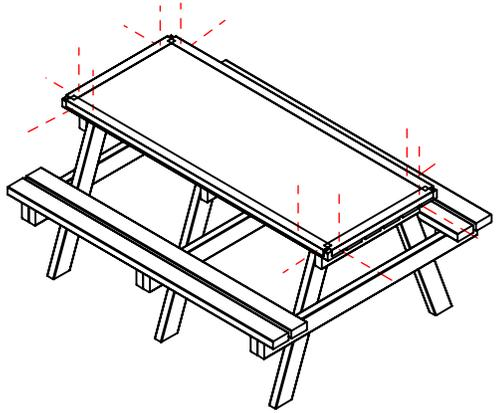
**Step 2** - Attach the corner caps by drilling and screwing through into the sides of the tabletop.
