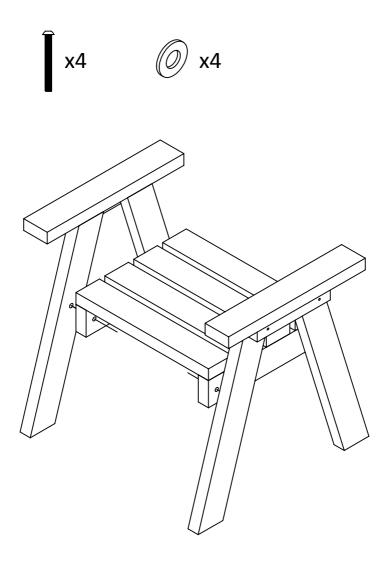
Step 2 Use remaining M10x60 bolts to secure Back Rest to Leg Assembly as shown in diagram.
