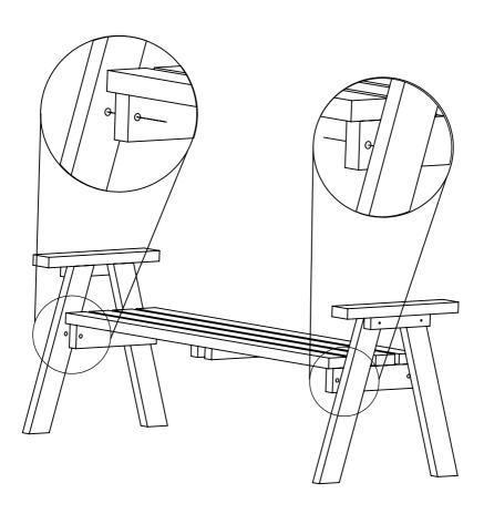
**Step 2** Screw Middle Legs to the seat, 2 screws per leg.
