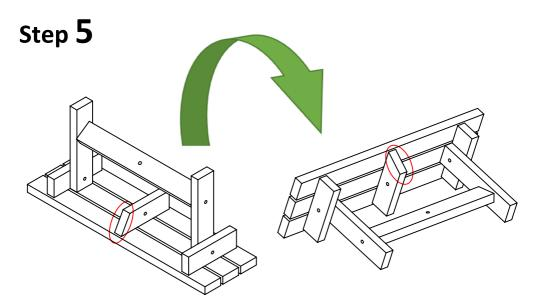
Flip the seat onto its side, with angled support strut facing upwards.
