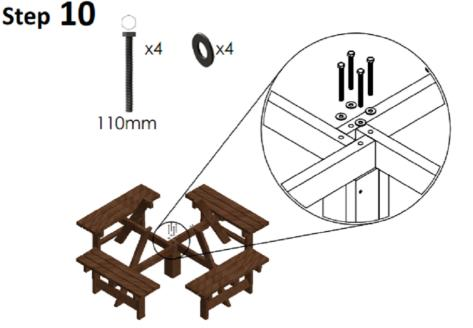
Tighten nuts and bolts with Spanner.
