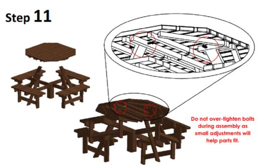
Carefully place Table Top onto Legs ensuring holes and supports align as shown.
