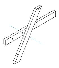
Do not over-tighten bolts during assembly as small adjustments will help parts fit.
