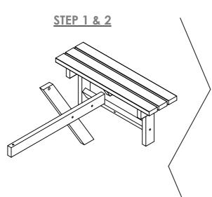
Bolt step 1,2 & 3 assemblies together using 90mm & 130mm bolts.
