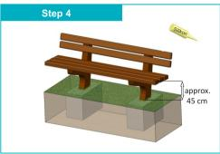
Set the bench in a concrete foundation and fix it while drying. Do not use while drying.
