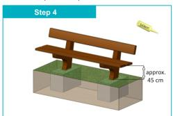
Set the bench in a concrete foundation and fix it while drying. Do not use while drying.
