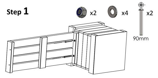
Lay the box end with the opening facing away from you, hold the seat into position with the holes lining up and bolt the two parts together using the Allen key and spanner,
