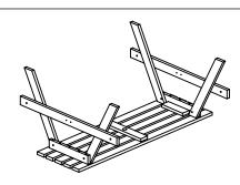
Step 2: With at least two people, flip the table the right way up and bolt the seats into the a-frames.
