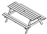
Step 3: Flip the table again and screw the diagonals into the a-frame crossbars and the middle table support.
