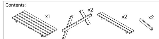
**Fixings** QTY M10x80mm Bolt M10 Nut 8 M10 Washer 16 50mm Wood 8 Screw
