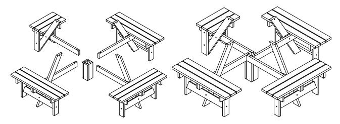
**Step 4:** Move the tabletop into position and bolt through the legs using x4 M10x120 Bolts.
