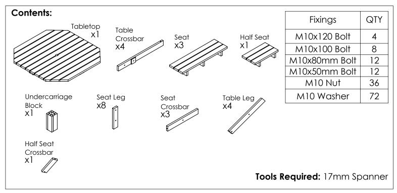
**Step 1:** Assemble the seat frames using 100mm, 80mm and 50mm bolts, bolting the seat legs together with the table crossbar, and into the seat. Bolt the table leg to the table crossbar then bolt into the seat undercarriage. Repeat x3.
