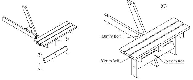
**Step 2:** Assemble the half size wheelchair seat using same method as previous seats.
