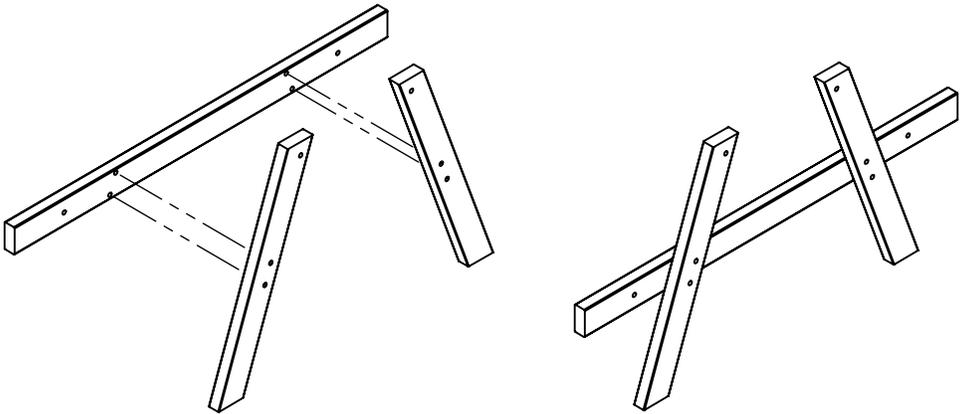
**Do not over-tighten bolts during assembly as small adjustments will help parts fit.**
