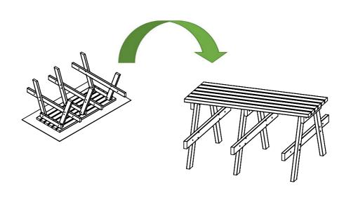
**Step 5** Place seats on A-Frames and fasten with bolts supplied.
