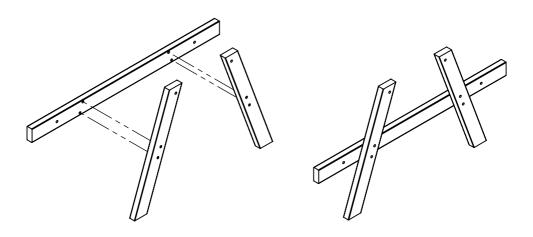
Do not over-tighten bolts during assembly as small adjustments will help parts fit.
