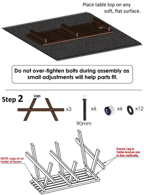
Fully tighten nuts and bolts with spanner and allen key.
