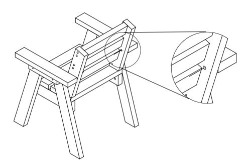
Step 3 Take Back Rest and line the front edge with the rear Seat slat. With Back Rest in position fix in position seen below.
