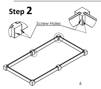
With the planks placed into the corner posts & the central posts, install the supplied screws into the screw holes on the corner posts & central posts.
