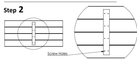
Once the support batton is located on the planks, please install the supplied screws through the support batton into the planks. Please repeat this process for the appropriate planks & support battons.
