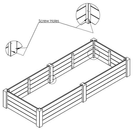
With the planks/plank assemblies placed into the corner posts & the central posts, install the supplied screws into the screw holes on the corner posts & central posts.
