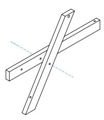
Bolt leg UC5 to UC1 using 90mm bolts supplied, repeat for all other legs.
