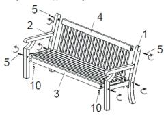
STEP 4: Check bench is stable and secure after all the bolts have been tightened
