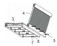
STEP 3: Assemble the backrest (4) and bench seat (3) with the left arm (1) and the right arm (2) Then tighten with bolts (5) as the image below shows
