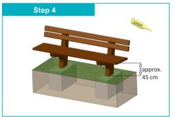
Set the bench in a concrete foundation and fix it while drying. Do not use while drying. Fill the screw head at the backrest with silicone.
