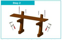
Place the seat element on the feet. Fit the connecting irons on the seat into the recesses of the bench feet and fix it with screws (5x60 mm).
