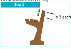
Place the backrest on the feet and fix it with the screws by using the predrilled holes. 2 screws per bench board (6x120 mm).
