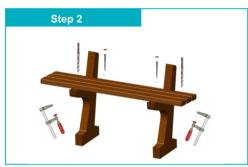
Place the seat element on the feet. Fit the connecting irons on the seat into the recesses of the bench feet and fix it with screws (8x70 mm) after placing an O-ring.
