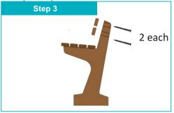
Place the backrest on the feet and fix it with the screws by using the predrilled holes. 2 screws per bench board (6x120 mm).
