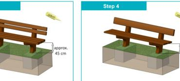
Set the bench in a concrete foundation and fix it while drying. Do not use while drying.
