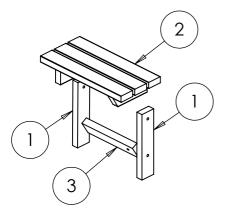
Assemble half seat as below, using (1x) 90mm bolt & (2x) 60mm bolts.
