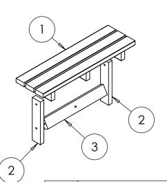
Assemble seats as below using (2x) 90mm & (2x) 60mm bolts supplied.
