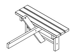
Bolt step 1 & 2 assemblies together using (1x) 90mm & (1x) 60mm bolts per seat.
