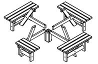
Secure seat assemblies to the block using (4x) 110mm bolts.
