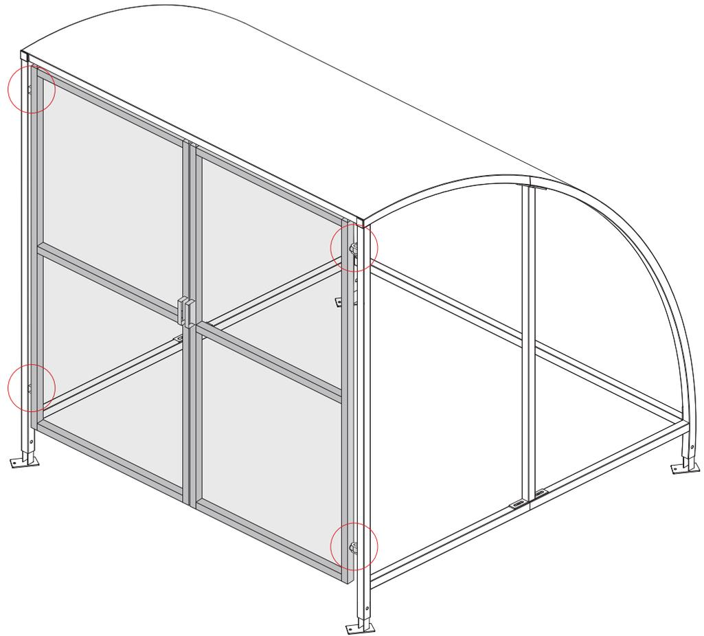
**!** Screw **SGH** Gate Hinge into the boss on the **LHG/RHG** Doors. Place the hinge into the brackets on the **LCSF/RCSF** Frames pushing **Pin** through the bracket hole using the **Nut** to hold in place. The doors can be adjusted by turning the **Boss Nut** accordingly.
