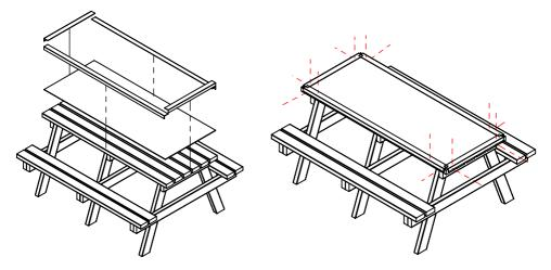
**Step 2** - Attach the corner caps by drilling and screwing through into the sides of the tabletop.
