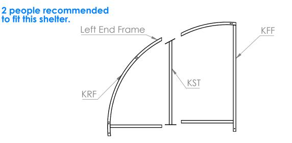
Note: Shelter ends have 2 sides Left and Right. Make sure all holes are in correct position before assembling.
