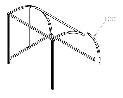
**Step 4** Repeat **Step 1, 2 and 3** with the opposite side of the shelter this time securing all centre bolts tightly making one complete unit.
