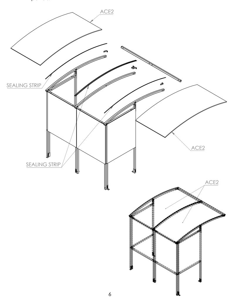
**Step 4** Apply sealing strips to the top of the panel and use **RC2** strips to cover the gap in the centre and the edges. Finish of the shelter by attaching the A1 angle trim.
