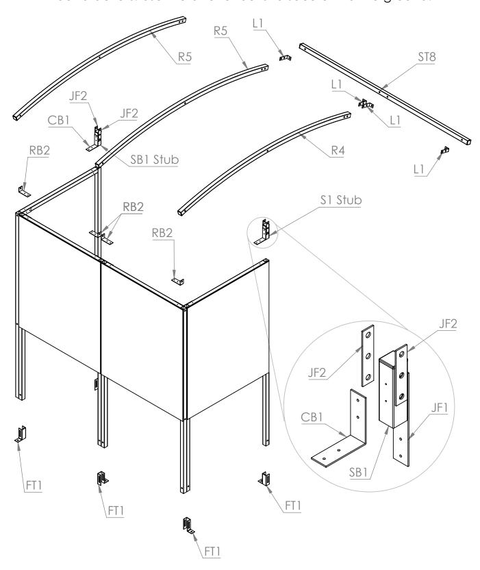
**Step 3** Apply sealing strips to rafters. Align the two **ACE2** roof panels with the outer edges of the shelter, leaving a gap in between the panels.
