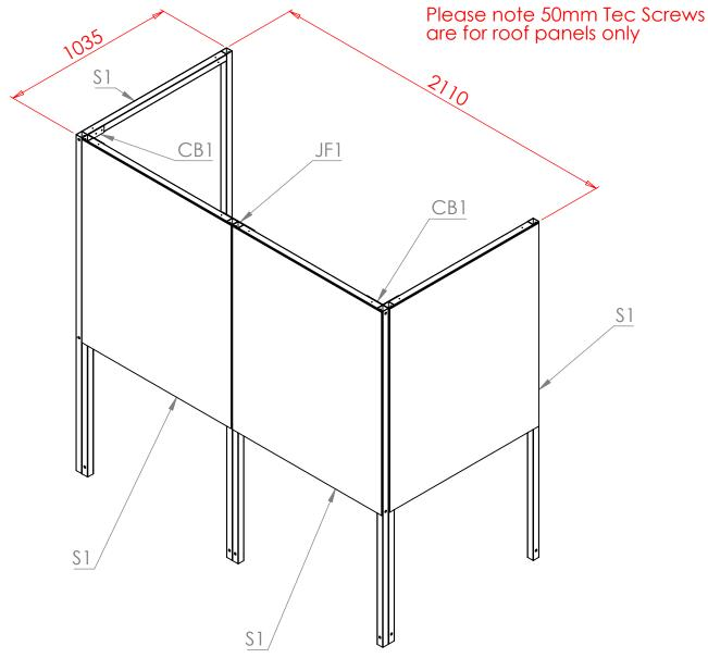
check shelter dimensions to ensure correct alignment
