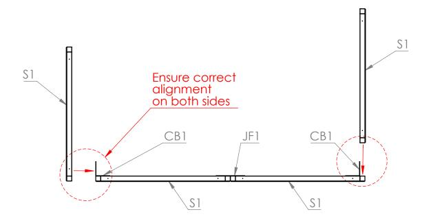
Step 2 Attach JF2 brackets to SB1 Stubs. Using CB1 and JF1 brackets secure SB1 to frame. Now fix the RB2 brackets to the rear of the frame, attach R4 & R5 rafters. Use L1 brackets to attach ST8 tie bar. Move the shelter in to its final position, make sure its square and attach FT1 foot brackets. Use the anchor bolts to secure it to the ground.
