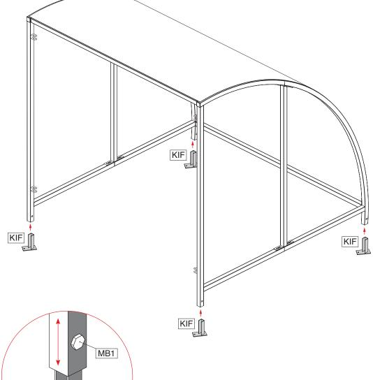
Move shelter to desired position and place **KIF** Foot into each leg. Adjust the shelter until level then drill through the foot and secure with MB1 Bolts.
