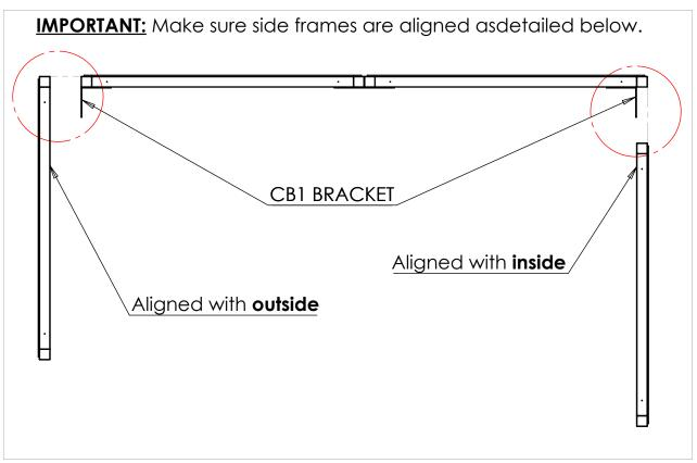
**Step 2** Attach front **\$1** frame and **\$T1** tie bar using **CB1** brackets in the corners and **JF1** brackets on the straight joints. Once the main structure is bolted together, move the shelter into its final position and install foot brackets **FT1** and **FT3** to secure shelter to the ground.
