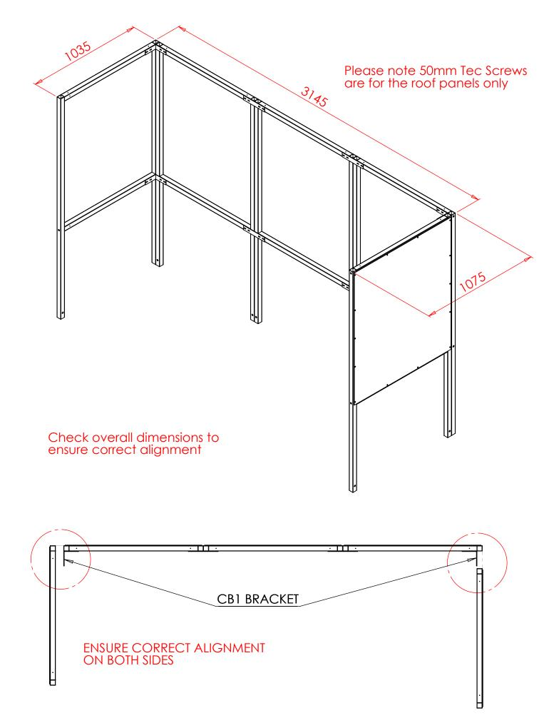
Step 2 Attach ST1 Roof Tie and Final S1 to the structure using CB1 and JF1 Brackets
