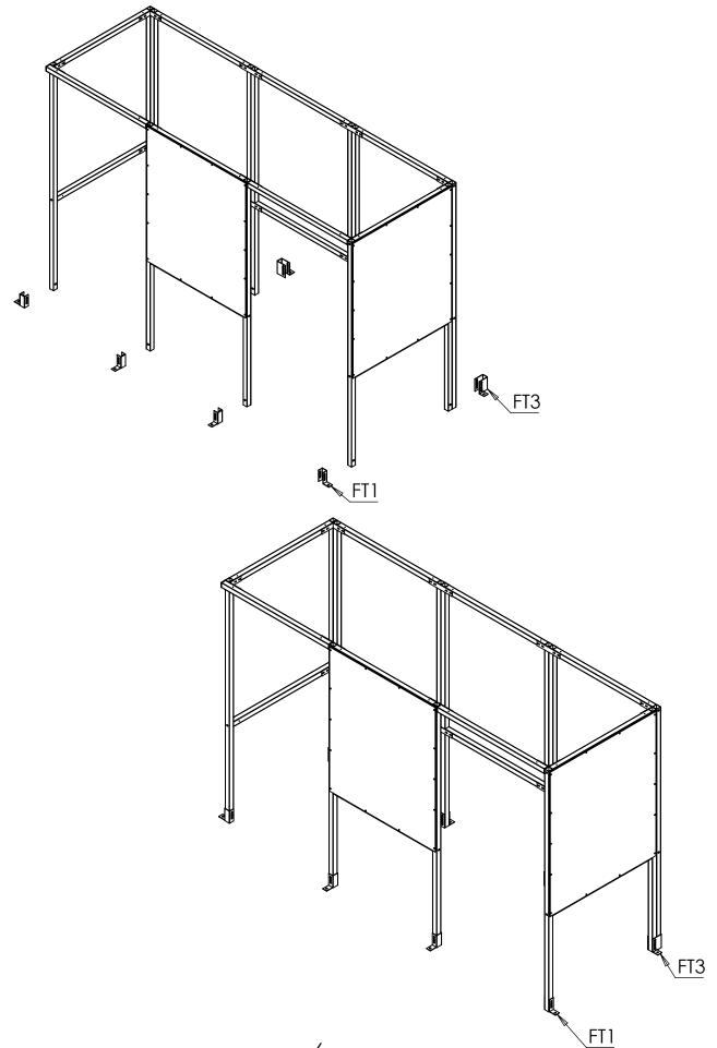
Step 4 Screw RB1 Brackets to the top of the frame and bolt R1 Rafters to framework.
