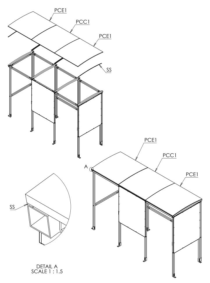
**Step 6** Secure panels in place using an **RC1 Strip** and **50mm Tech screws**, then attach the **2MD** Edge Trim to the outer edges of the panels. Then fit the black plastic caps on exposed nuts and bolts. Fit the square plastic end caps to any open ends of box sections.
