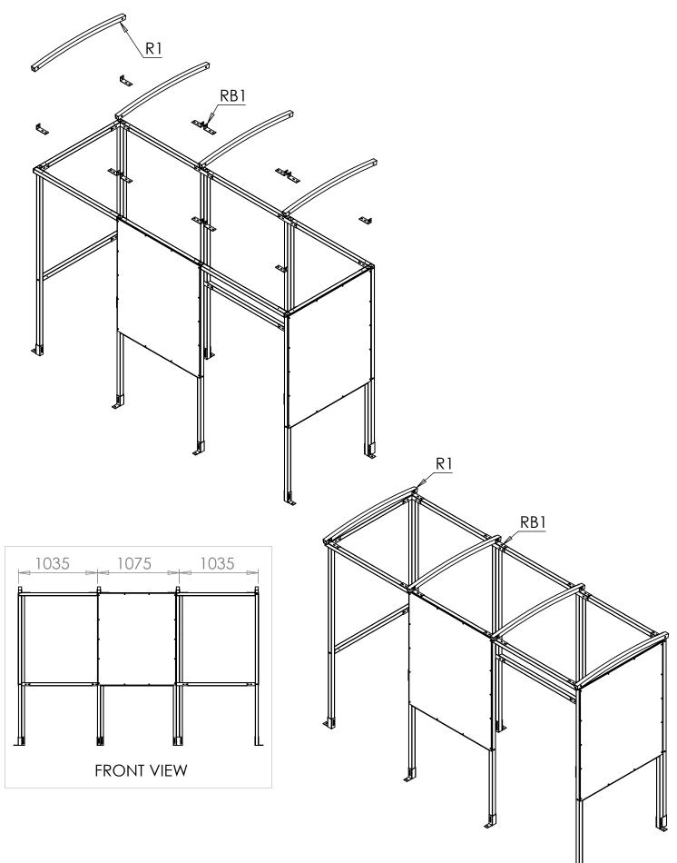
**Step 5** Attach two **Sealing strips** to the top of each rafter then place **PCE1** and **PCC2 Panels** on top of the strips leaving a small gap between each. Apply more sealing strips to the top of the roof panels, directly above the first strips.
