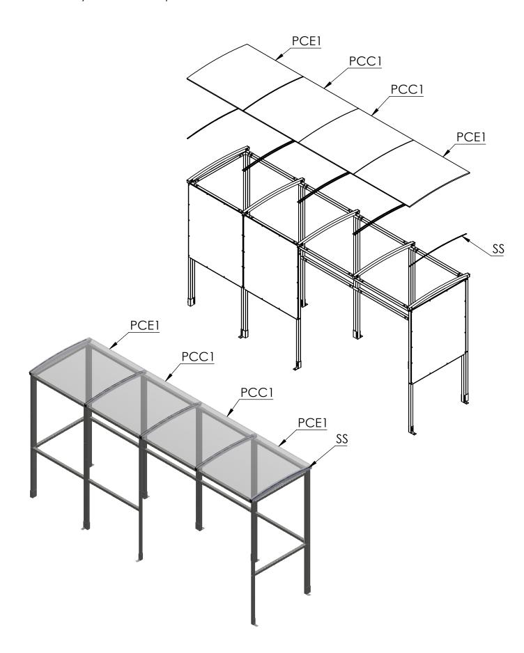
**Step 4** Secure the roof panels in place by drilling the **RC1** strips directly into the frame of the shelter using the **Tech 50 screws.** Then apply the **2MD** edge trim along the bottom edges of the roof. Push fit the Black plastic caps on exposed nuts and bolts. Use a mallet to fit the square plastic end caps to any open ands of box sections.
