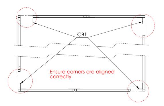
**Step 2** Move shelter in to its final position, make sure everything is square and secure to the floor using **FT1** and **FT3** foot brackets.
