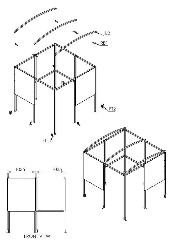
**Step 3** Apply **SS** sealing strips to the rafters (two for cental rafter) and line up the **PCE2** roof panels to the outside of the shelter, leaving a gap between them. Apply more sealing strips to the top of the roof panel directly above the first strips.
