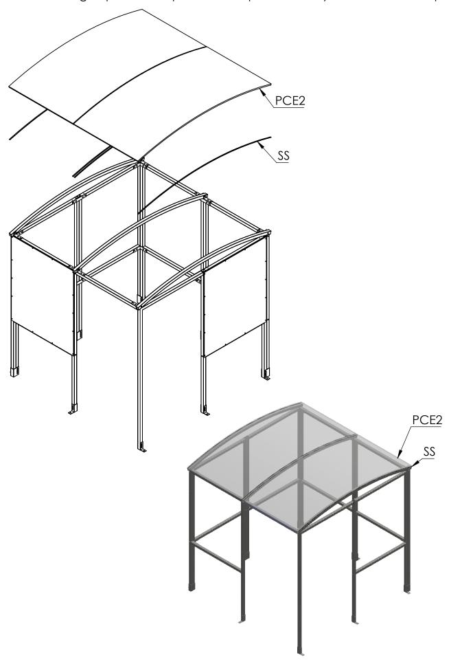
**Step 4** Apply **RC2** strips on top of the panels and use **50mm Tech screws** to secure them in place. Then clip on the **2MD** edge trim to the bottom of the roof panels. Then fit the Black plastic caps on exposed nuts and bolts. Fit the square plastic end caps to any open ends of box sections.
