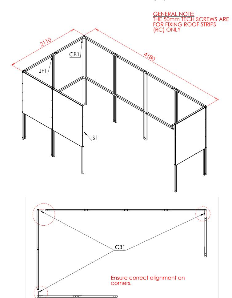
**Step 2** Attach **P1** post using one **JF1** bracket, then attach **ST3** tie bar using another **JF1** bracket and two **CB1** brackets.
