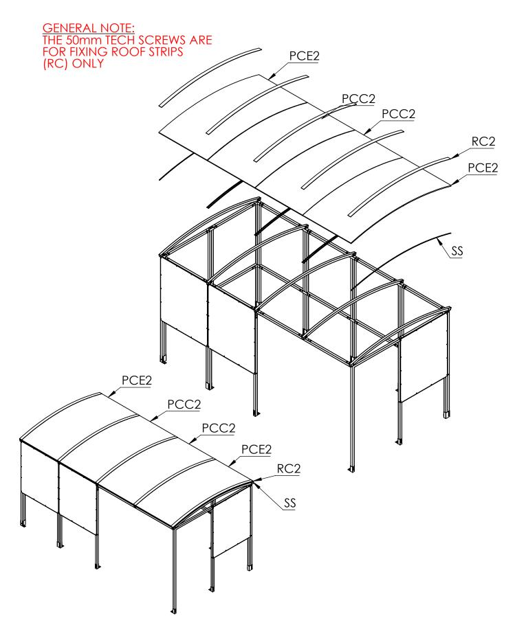
**Step 5** Clip on the **2MD** end caps. Then fit the Black plastic caps on exposed nuts and bolts. Fit the square end caps to any open ends of box sections.
