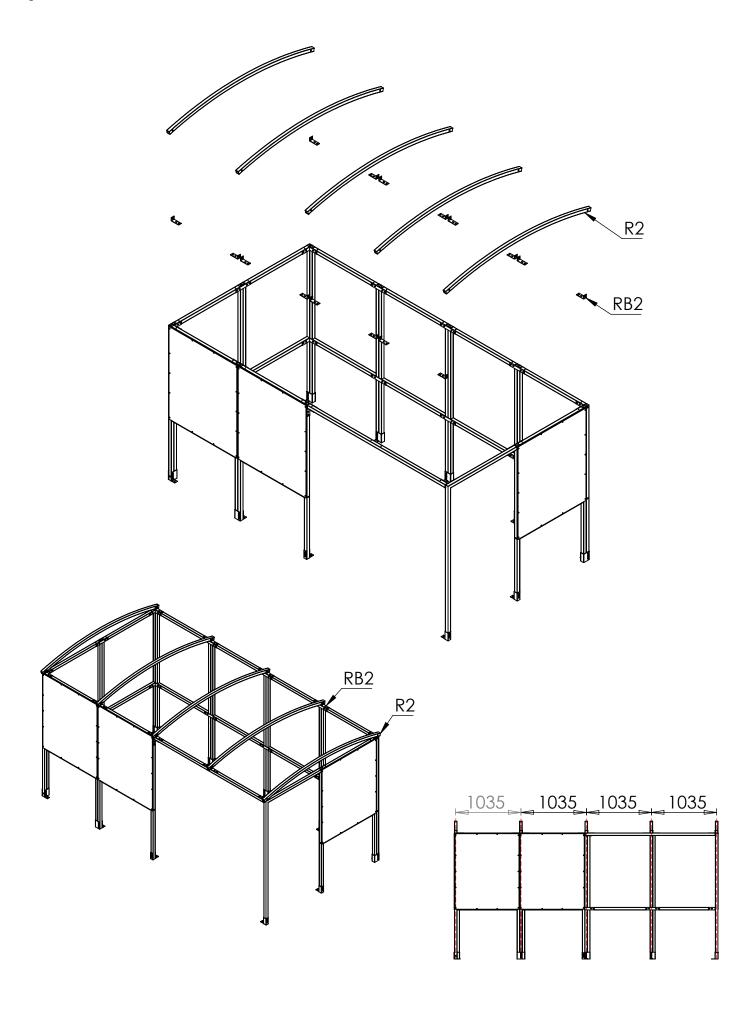
**Step 4** Apply sealing strips **(SS)** to the top of the rafters. Align **PCE2** roof panels with the outer rafters then space out the **PCC2** panels evenly. Apply more **SS** strips to the top of the roof panels, directly above first strips. Cover the two edges along the outer rafters and gaps with **RC2** strips before screwing them into place using the **50mm TEC screws**.
