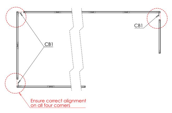
**Step 2** Attach **P1** Post using one **JF1** bracket then attach **ST3** Tie bar using two **CB1** brackets and one **JF1** bracket.
