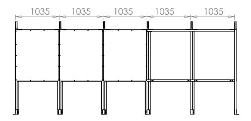
**Step 4** Attach **PCC2** roof panels and **PCE2** roof panels on top of the sealing strips. Apply more sealing strips to the top of the roof panels directly above the first strips Screw down the **RC2** strips to cap it and seal off the end of the panels with the **2MD** end caps. Then fit the Black plastic caps on exposed nuts and bolts. Fit the **EC40** square end caps to any open ends of box sections.
