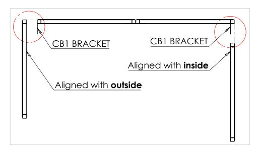
**Step 2** Insert **EC40** end caps into both ends of the **ST1** tie bar. Attach front **S1** frame and **ST1** tie bar using **CB1** brackets in the corners and **JF1** brackets on the straight joint. Once the main structure is secured, move the shelter into its final position and install foot brackets **FT1** and **FT3** to fix shelter to the ground.
