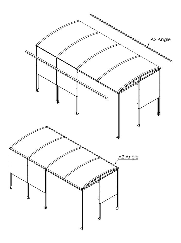
**Plan view**Suggested size for concrete base: 200mm / 7.87in oversized on all four sides.
