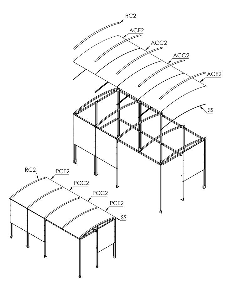
**Step 5** Fit the square end caps (**EC40**) to any open ends of box sections. Screw **A2** roof angles onto the edges of the roof as shown below.
