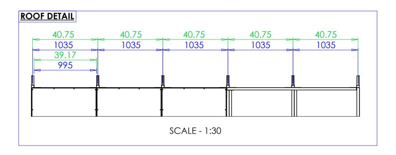
**Step 4** Attach **ACC2** roof panels and **ACE2** roof panels on top of the sealing strips. Screw down the **RC2** strips, along the gaps in the panels. Screw down the **A2** end caps along the edges of the shelter. Then fit the Black plastic caps on exposed nuts and bolts. Fit the **EC40** square end caps to any open ends of box sections.
