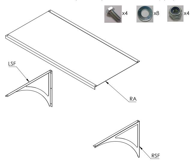
**Step 2** Another person will be required to attach the canopy to the wall. It helps to hold and level the canopy in the desired position before marking and drilling the holes in the wall.
