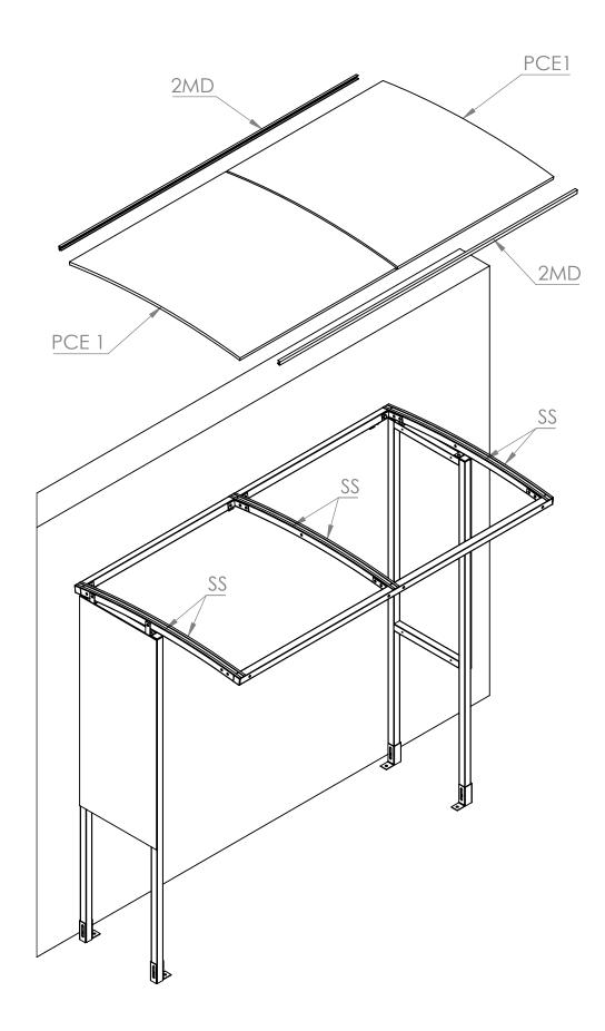
Step 6 Apply six more SS sealing strips to the top of the roof sheet and line them up with the ones underneath. Then align the RC3 roof strips and use 50mm Tec screws to secure them.
