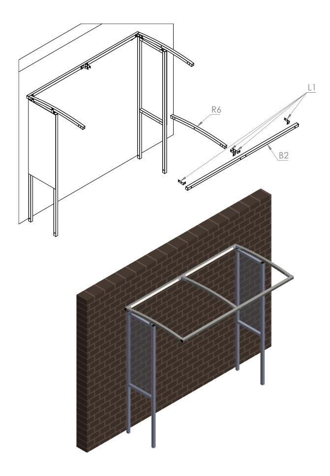
Step 4 Make sure the shelter is square before attaching the FT1 floor fixing brackets.
