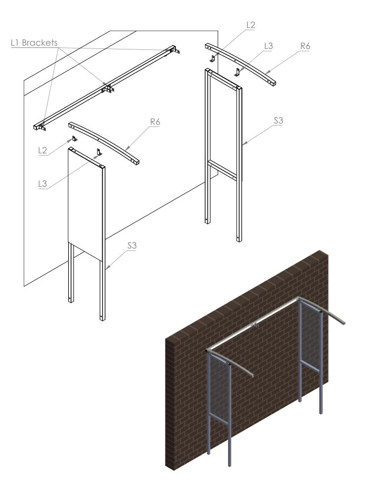
**Step 3** Use two L1 brackets to secure the front beam (B2). Also attach the Central rafter (R6) using four more L1 brackets.
