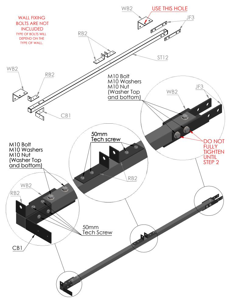
**Step 2** Fix the the same brackets from step one to the **ST13** tie bar as below. Attach the completed rear tie bar to the two **S3** frames. The shelter can now be moved into its final position, squared up and attached to the wall. Four foot brackets **FT1** can then be attached to the bottom of the legs.
