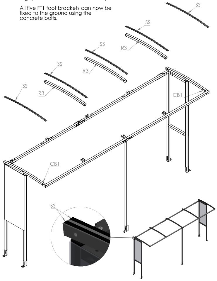
**Step 5** Place the roof sheets in their position, The **RC1** sheets are to be lined up with the edge of the shelter and the **RC2** sheets are to be spaced in the center. Then attach the **25A** roof angle and use the 50mm Tec screws to fix the roof sheets and angle into place. (DO NOT ATTACH ROOF SHEETS TO THE RAFTERS UNTIL STEP 6)
