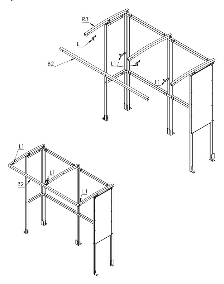
**Step 4** Apply sealing strips to **R3** rafters then put the **PCE1** Panels on top, apply more sealing strips on top of the panels and secure down with **RC1** strips, screwed into the rafters with **50mm Tech screws**. Then attach the **2MD** edge trim.
