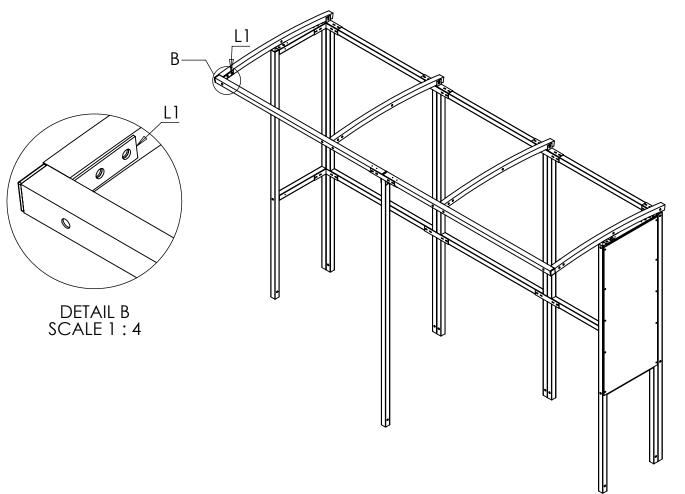
**Step 4** Attach the **FT1** and **FT3** foot brackets, Move the Shelter into its final position and make sure its square. Then use concrete anchor bolts to secure it to the the ground.
