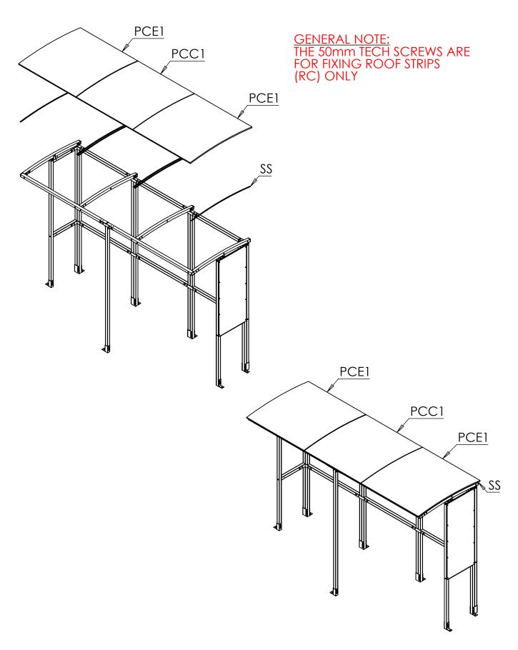
**Step 6** Attach the **RC1** roof strips, screwing directly into the rafters using **50mm Tech Screws.** Push on the **2MD** edge trim. Then fit the Black plastic caps on exposed nuts and bolts. Fit the square end caps **(EC40)** to any open ends of box sections.
