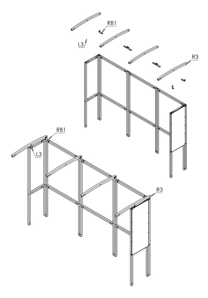
**Step 3** Assemble the **B3**'s and P1 using the JF1 and RB1 brackets as shown below. Attach front beams **(B3)** and centre post **(P3)** to the rafters using the L1 brackets.
