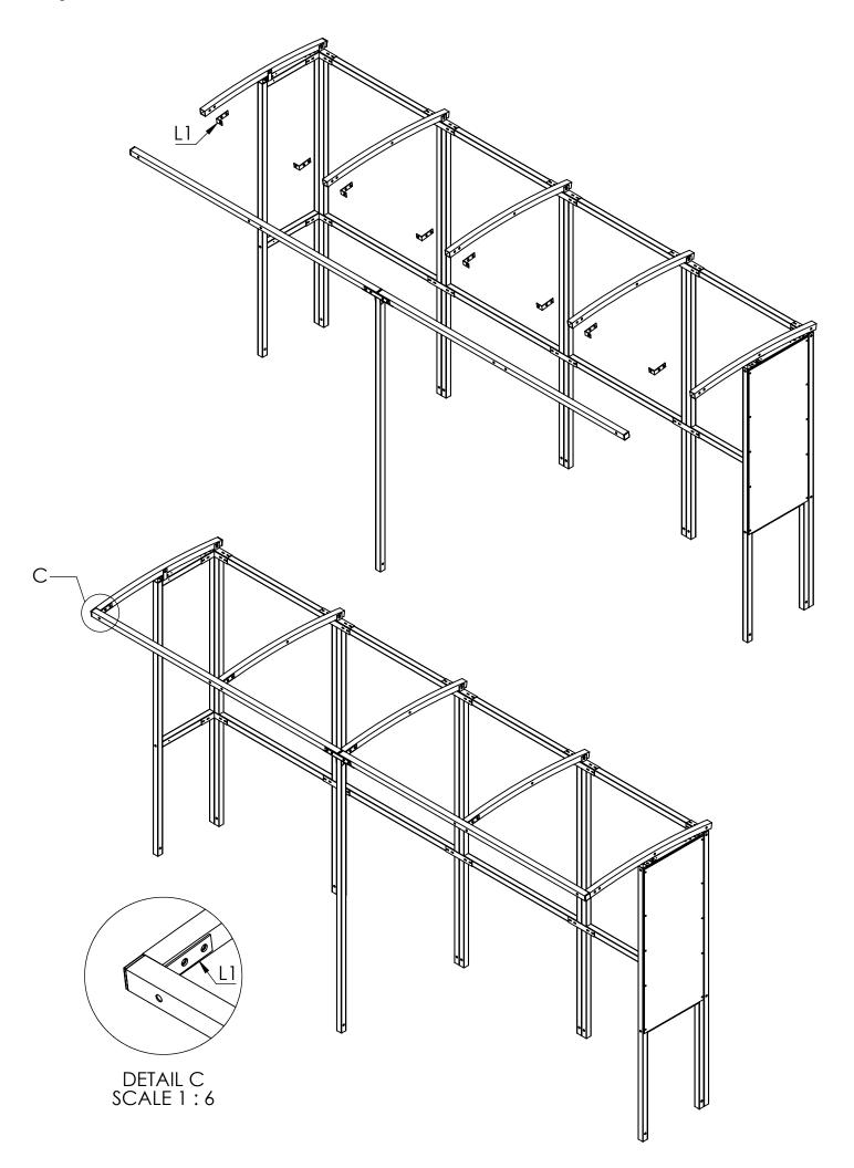
**Step 5** Move the shelter to its final position and make sure it is square and level. Then attach the **FT1** and **FT3** foot brackets and use anchor bolts to secure the structure to the ground.
