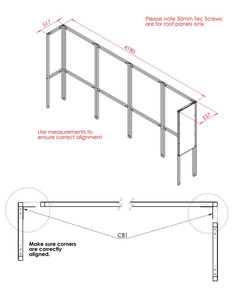
**Step 2** Attach the **R3** end rafters using **L3** brackets at the front and **RB1** brackets for the rear.
