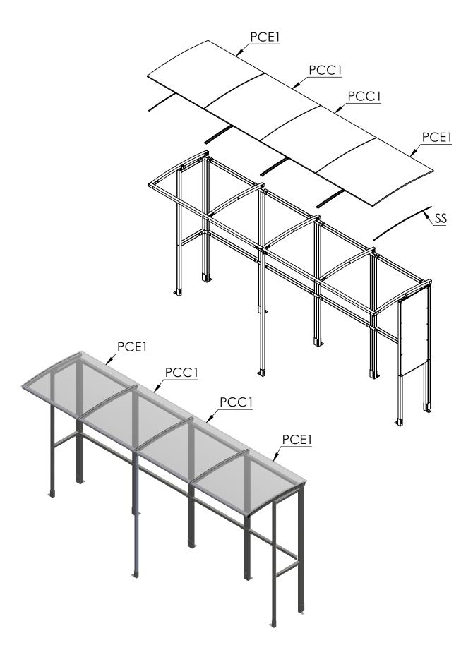
**Step 7** Screw down the **RC1** strips using the **50mm Tech screws** to secure the roof panels in place. Then push the **2MD** edge trim on to the bottom edge of the roof panels. Fit Black plastic caps on exposed nuts and bolts and fit the square plastic end caps to any open ends of box section.
