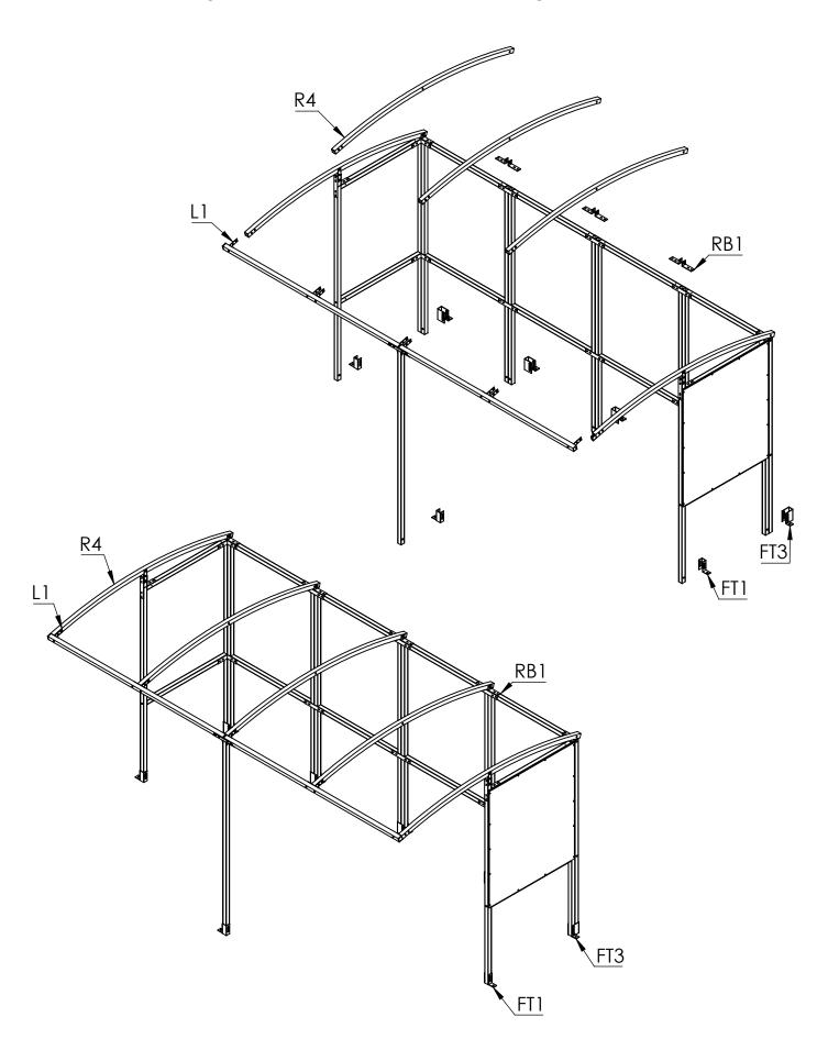
**Step 5** Stick the sealing strips (**SS**) to the rafters and line up the **PCE2** panels with the outside of the shelter then equally space the **PCC2** panels in the gap. Apply more sealing strips on the top of the roof panels directly above the strips on the rafters.
