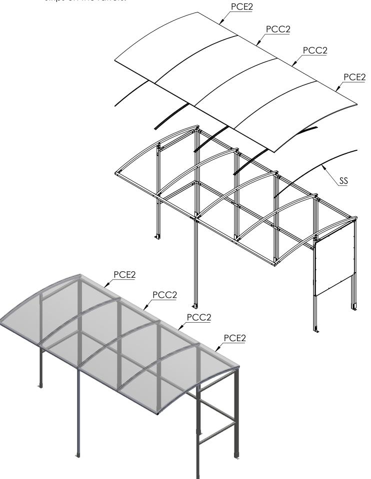
**Step 6** Screw down the **RC2** strips into the rafter with the **50mm tech screws** to secure the roof panels and push the **2MD** end caps on the bottom of the panels.
