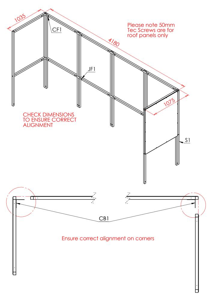
**Step 2** Attach the **S1 stubs** to the front of the frame using **CB1**, **JF1** and **JF3** brackets, then bolt the **R4** and **R5** rafters into place using the **RB1** brackets and the stubs
