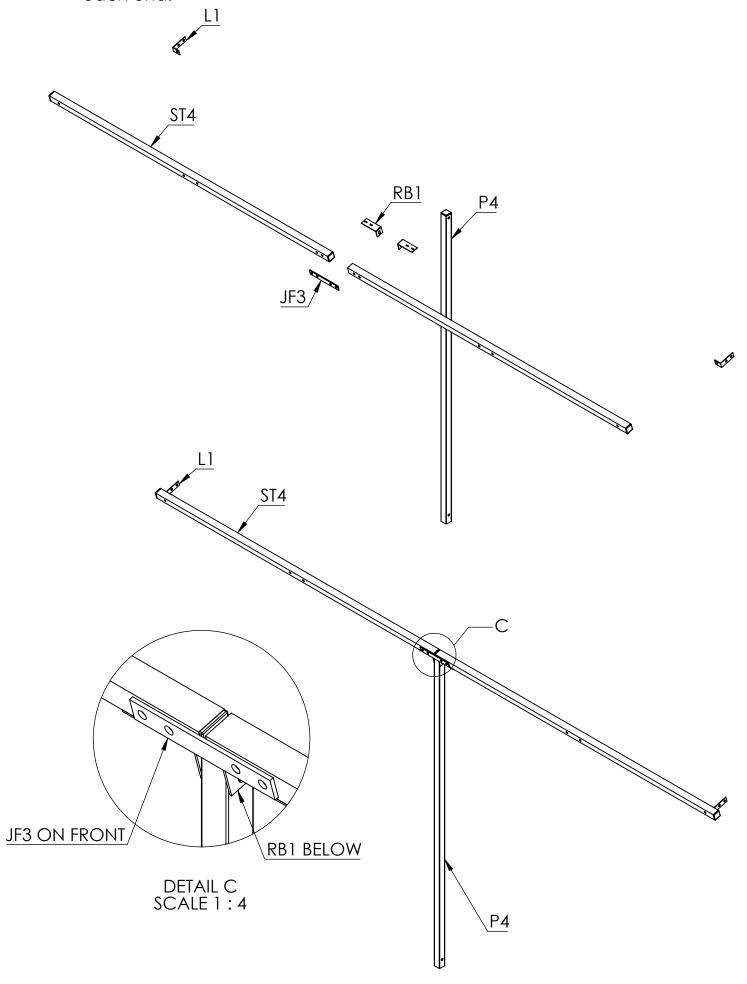
**Step 4** Attach the T-section to the shelter, then fix the **R4** rafters in place using more **RB1** brackets on the rear and **L1** brackets on the front. Bolt the **FT1** and **F3** brackets to the shelter and move it to its final position before using anchor bolts to secure it to the ground.
