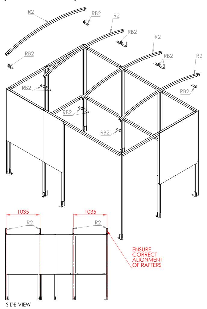
**Step 4** Stick sealing strips (**SS**) to the rafters. Align the **PCE2** roof panels with the outer roof rafters and equaly space the **PCC2** panel in the middle.
