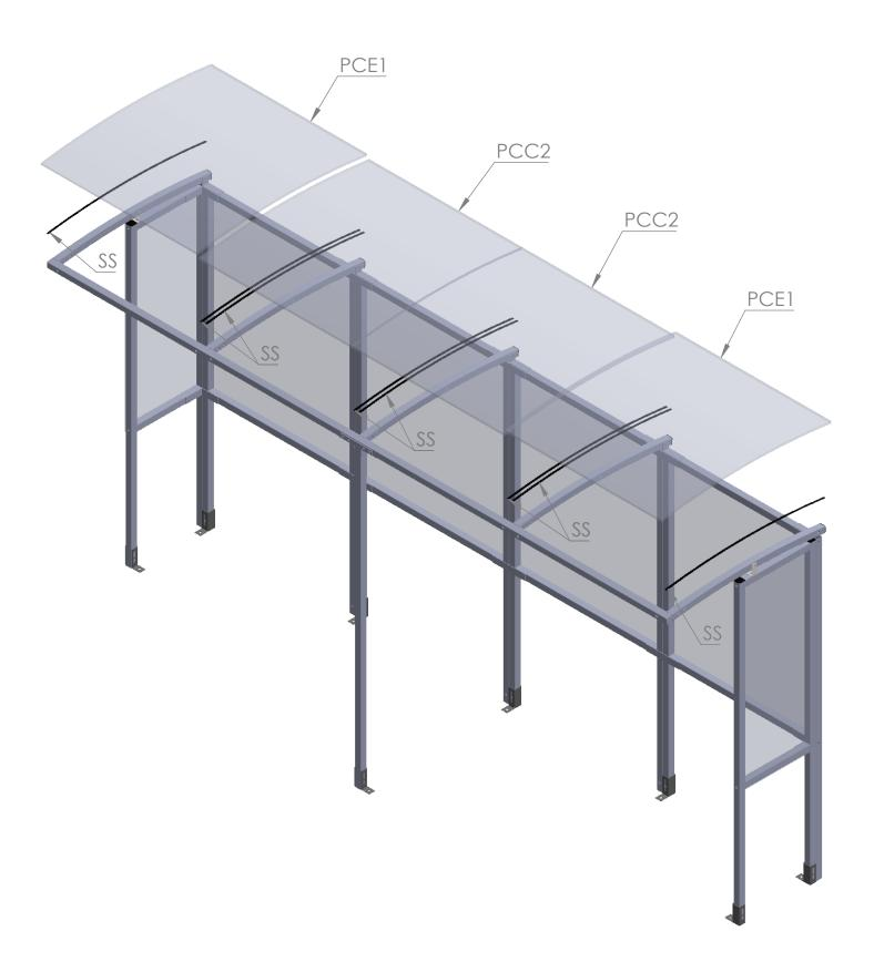
**Step 7** Screw down the **RC1** strips to secure the roof panels in place. Then push the **2MD** edge trim on to the bottom edge of the roof panels. Fit Black plastic caps on exposed nuts and bolts and fit the square plastic end caps to any open ends of box section.
