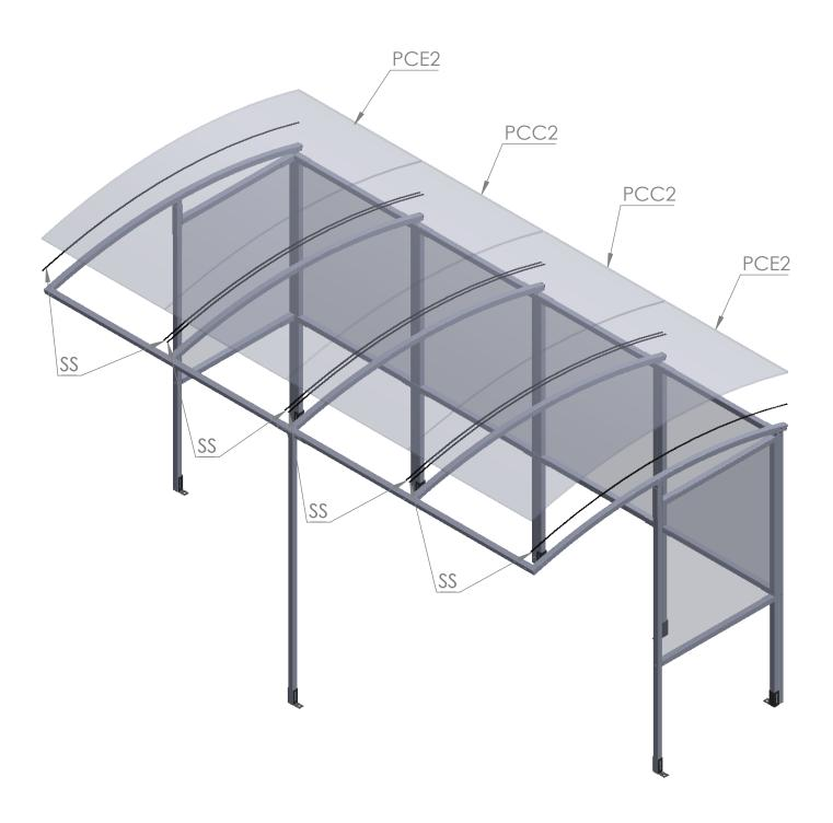
**Step 6** Screw down the **RC2** strips to secure the roof panels and push the **2MD** end caps on the bottom of the panels.
