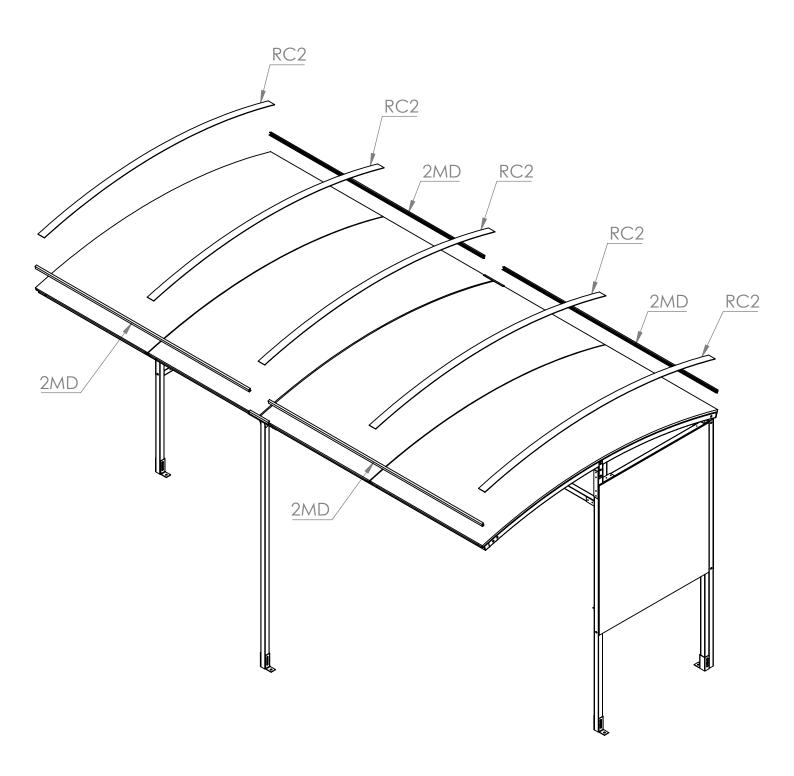
**Step 7** Attach the **FT1** brackets to the shelter and move it to its final position before using anchor bolts to secure it to the ground.
