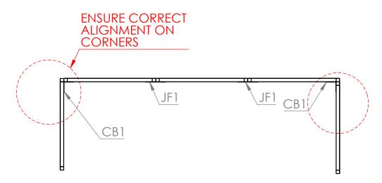
**Step 2** Use **JF1** and **CB1** brackets to attach the **S1** frame and **ST1** Tie bars.
