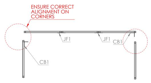
**Step 2** Use **JF1** and **CB1** brackets to attach the **S1C** frame and **ST1** Tie bars.
