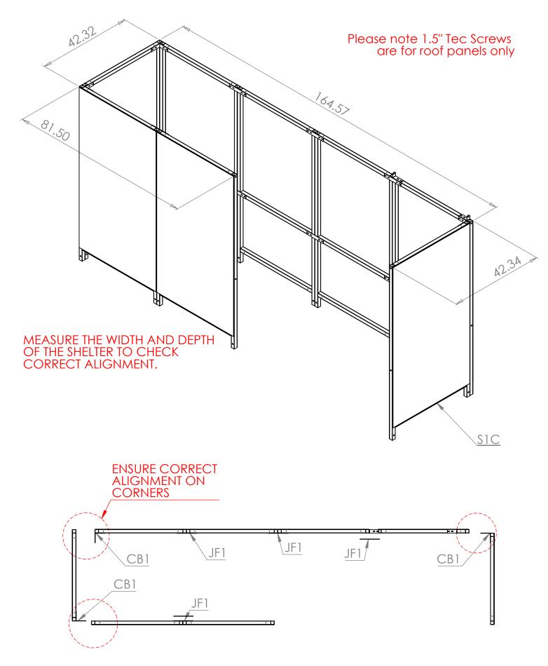
Step 2 Use JF1 and CB1 brackets to attach the S1C frame and ST3 Tie bar.
