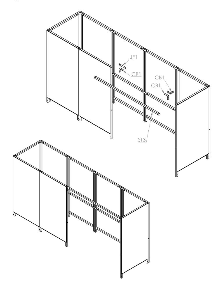
**Step 3** Attach **AR1R** rafters using **DR** brackets. Secure the **AR1IS END PANELS** to **S1C** frames using tec screws. The end rafters need to be placed in position at the same time as the **END PANELS**.
