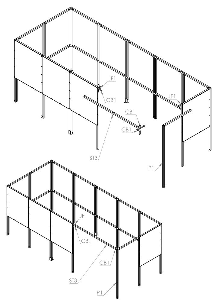
**Step 3** Attach **AR2R** rafters using **DR** brackets. Secure the **AR2IS** end panels to **\$1** frames using tec screws. The end rafters need to be placed in position at the same time as the **AR2IS** end panels. Stick sealing strips to each rafter.
