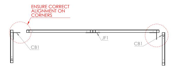
**Step 2** Attach **ST15** Tie bars to **S3C** frames using **CB1** Brackets. Assemble the **ST15** Tie Bars with the **ST3** Tie bar and the **P5** Post, using the **CB1** Corner Brackets and the **JFT** Bracket as shown below.
