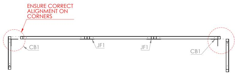
**Step 2** Attach **ST15** Tie bars to **SC3** frames using **CB1** Brackets. Fix the **ST5** Tie bars to the **ST15** bars using **CB1** Brackets and attach to the **P5** Post using the **JFT** Plate. Fix a **JF1** Bracket to the top of the two **ST5** Bars.
